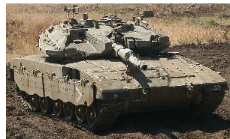
Sloped armour is armour that is mounted at a non-vertical and non-horizontal angle, typically on battle tanks and other armoured fighting vehicles.
