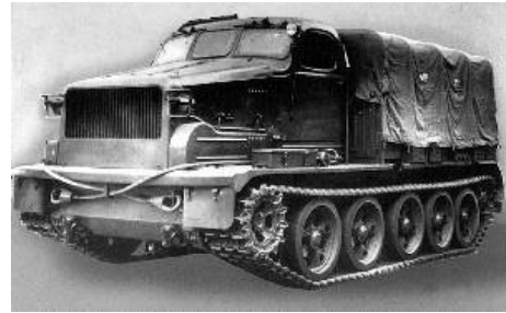
Artillery tractor is a kind of tractor, also referred to as a gun tractor, a vehicle used to tow artillery pieces of varying weights.
