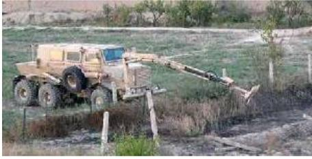
The Buffalo A2 is a heavily armored truck specifically designed to protect its occupants from mines and improvised explosive devices. The Buffalo is a recognized leader in the global mine-protected route-clearance vehicle class, with approximately 238 Buffalo A2 vehicles delivered to U.S. units throughout the world.
