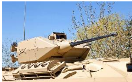
FNSS’ Brand New SABER 25mm One Man Turret successfully completes firing qualification tests on FNSS PARS 8x8 Infantry Fighting Vehicle.
