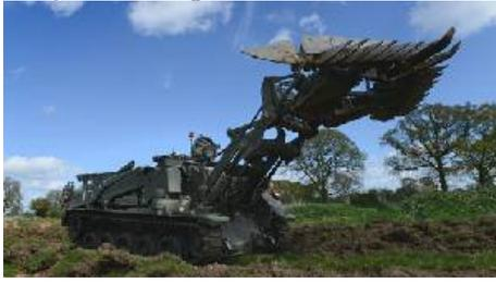
The vehicle has also been equipped with a long-reach rummage arm developed to probe and unearth suspect buried devices from a safe distance. On display at DSEI this week, these new developments are part of ongoing capability enhancements which further boost Terrier's ability to conduct route proving and clearance tasks.
