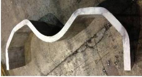
Aluminium armour materials were never developed with intent to be cold formed, and so intrinsically pose challenges to avoid common modes of failure such as cracking. We have created a reliable and repeatable cold forming process, backed by scientific and engineering validation. We have pushed our current forming technology to its limits, and the integrity of parts produced are validated using innovative and standardised methods of material testing to assure optimum material resilience.
