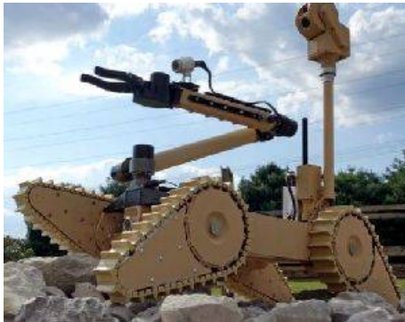
HUNTSVILLE, Ala. -- Northrop Grumman Corporation’s subsidiary Remotec Inc. is unveiling the newest member of the Andros line of proven unmanned ground vehicles (UGVs), the Interoperability Profile (IOP)-compliant Nomad.
