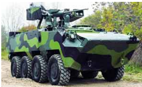
A special version equipped with a remote controlled weapon station (RCWS) cal. 30mm of Rafael.
