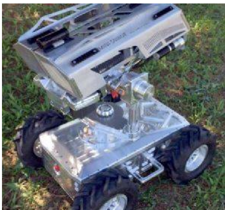
Developed on an unmanned ground vehicle, the robot, called Snibot, can shoot with high precision to its targets.
