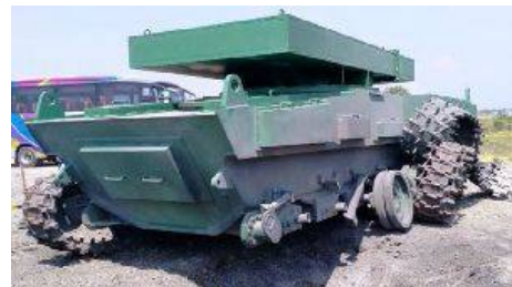
On July 12, 2018, the Indonesian company PT Pindad jointly with the Turkish company FNSS conducted a mine explosion test of the prototype of the medium tank.
