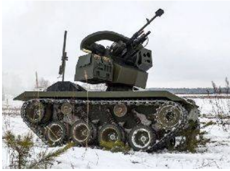
The Ministry of Defense of Russia has published video of testing the latest Russian Nerekhta Combat Unmanned Ground Vehicle (CUGV) which interacts with the fighters of motorized rifle units.
