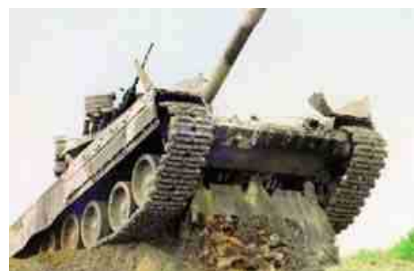
A small dozer blade attached to the front of an armored vehicle to enable the vehicle to dig itself in, in order to give better protection.
