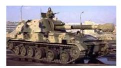
A self-propelled gun is a gun, whether it be an artillery piece, anti-tank gun, or anti-aircraft gun, mounted on a motorized wheeled or tracked chassis. As such the gun can be manoeuvred under its own power as opposed to a towed gun that relies upon a vehicle or other means to be moved on the battlefield. Self-propelled guns are combat support weapons; they are employed by combat support units fighting in support of, or attached to, the main combat units: infantry and armour.
