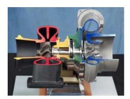
A turbocharger is an exhaust-gas driven forced induction device used in internal combustion engines to improve engine performance by forcing compressed air into the combustion chambers, allowing more fuel to be burned, resulting in a larger power output.
