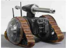
This portable, lightweight robot is operated by a single operator, and is designed to negotiate obstacles typical of an urban environment, such as climbing stairs and rubbles,
