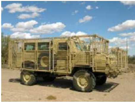
BAE Systems has installed the first two LROD(tm) rocket-propelled grenade (RPG) protection kits on U.S. Army RG31 and RG31A1 mine-protected vehicles.
