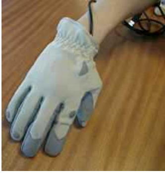
A new glove lets soldiers operate wearable computers while still holding their weapons.
