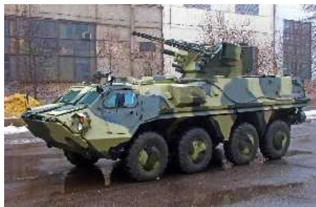
KMDB, the leader of the Ukrainian armoured construction, will demonstrate the latest variant of its BTR-4 APC with PARUS weapon station.
