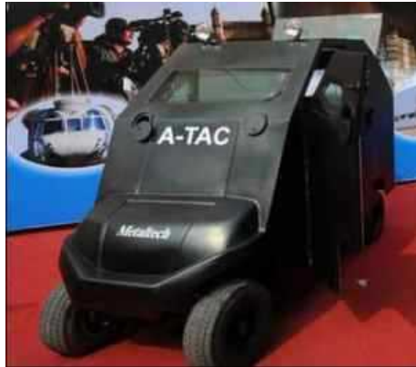
The battery operated, two million rupee ($45,000) Anti-Terrorist Assault Cart (Atac) is said to resemble a bullet-proof golf buggy with firing ports.
