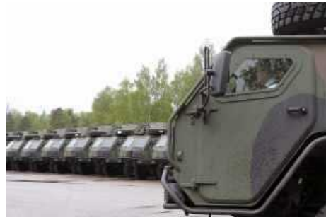
Delivered trucks are equipped with effective mine protection and feature a cabin of armour steel.
