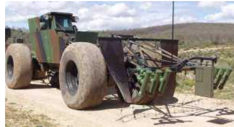
Development of SOUVIM 2, a mine path clearing system designed and manufactured by MBDA since 2008, has just been completed.
