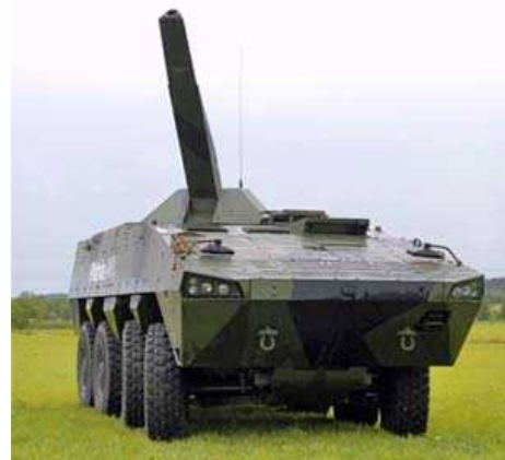
Patria Nemo 120 mm mortar system has been selected as one of the weapon systems for LAV II vehicles delivered by General Dynamics Land Systems - Canada as part of a Foreign Military Sales (FMS) project for the US Government.
