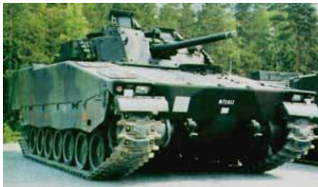
Ornskoldsvik, Sweden -- Two Norwegian Army CV9030 infantry fighting vehicles have been using rubber tracks in northern Afghanistan since December.
