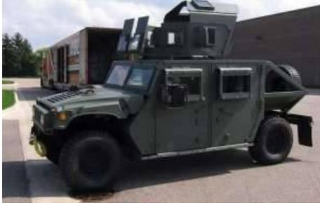
Capable of going from traditional canvas doors to a full "Frag Kit" protection level, this solution also incorporates a blast shield of advanced materials under the crew cab. The combination allows the Marine Corps to recapture the full weight savings needed to insure expeditionary amphibious operations and long term storage aboard ships.
