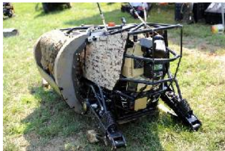
Two completed prototype robotic “pack mules” exhibit reduced noise, new gaits, and improved perception
