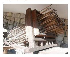
The hwacha consisted of a two-wheeled cart carrying a board filled with holes into which the singijeon were inserted.
