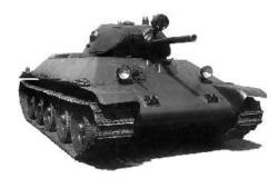
Medium tank was a classification of tanks, primarily used during World War II. The medium tank, as the name suggests, represented a compromise in features between the reconnaissance and mobility
