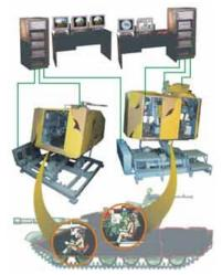
The practical skills in technical maintenance of units and systems of armoured vehicles can be acquired by trainees on operating training models which provide a full-scale simulation of the units and systems being studied.
